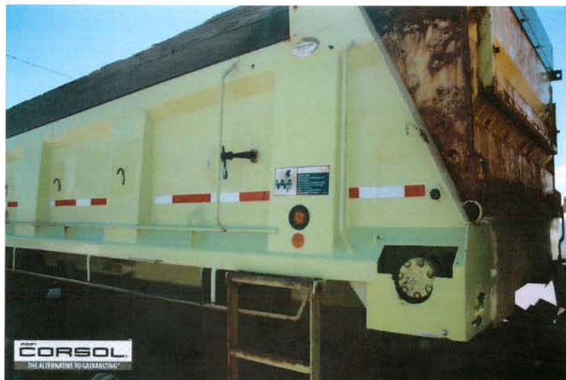
Unit 34. The front gate and the ladder were painted utilizing the WS DOT standard paint system
